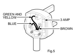
The wire which is coloured BROWN must be connected to the terminal which is marked with the letter 'L' or coloured RED.
